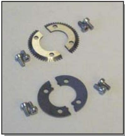
The perforator blades are split into two matching halves and are fitted to the drive wheels as shown in the photograph using the four screws supplied.
